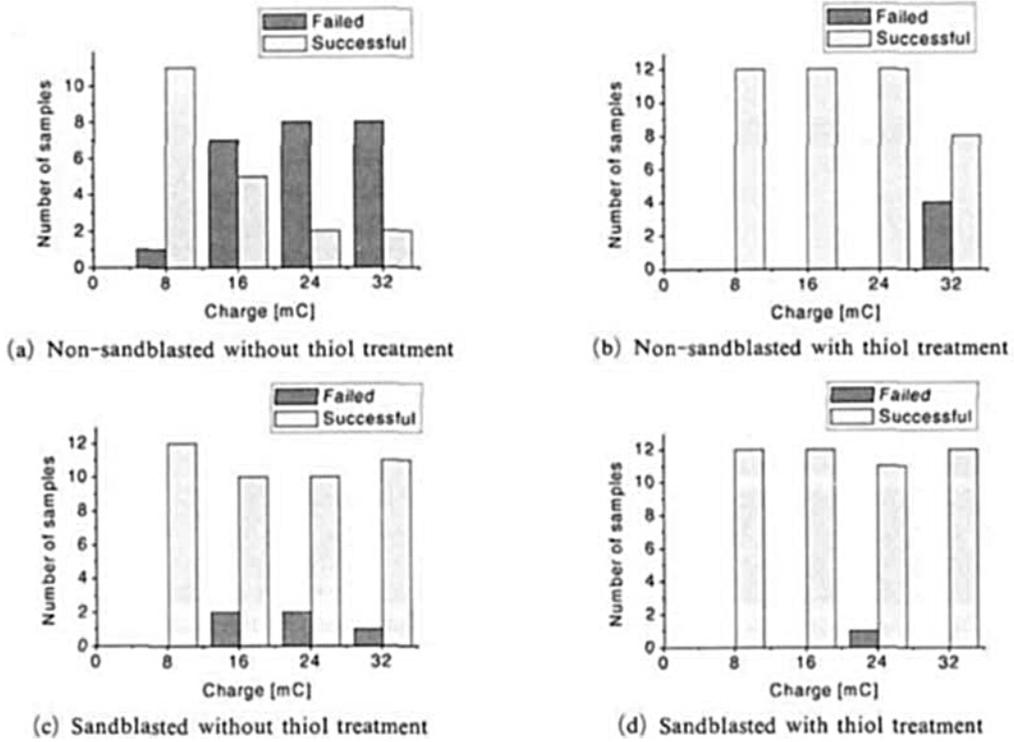
Fig. 8 Results of adhesion tests for each case with respect of applied charges (8, 16, 24, and 32 mC)
