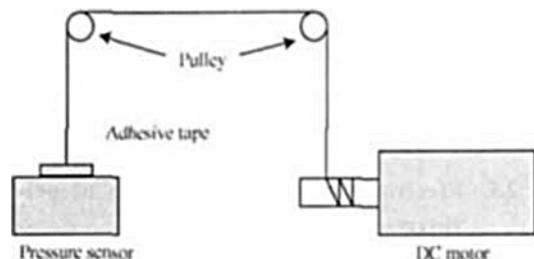
Fig. 3 Measurement of stripping-off force with pressure sensor
