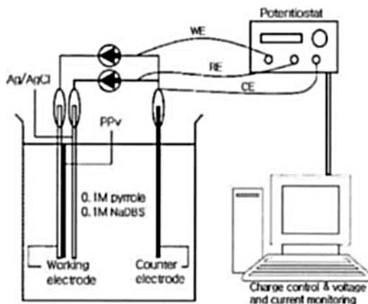
Fig. 2 Schematic of polypyrrole electrochemical polymerization system
